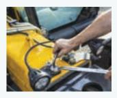
• Adjusting the telescopic boom pads has been simplified, a simple nut screw and lock nut system making adjustment quick and easy
