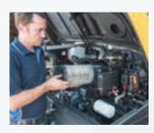
• The engine air filter is easy to check, clean or replace, without the need for tools The engine hood lifts on gas struts for full access.
