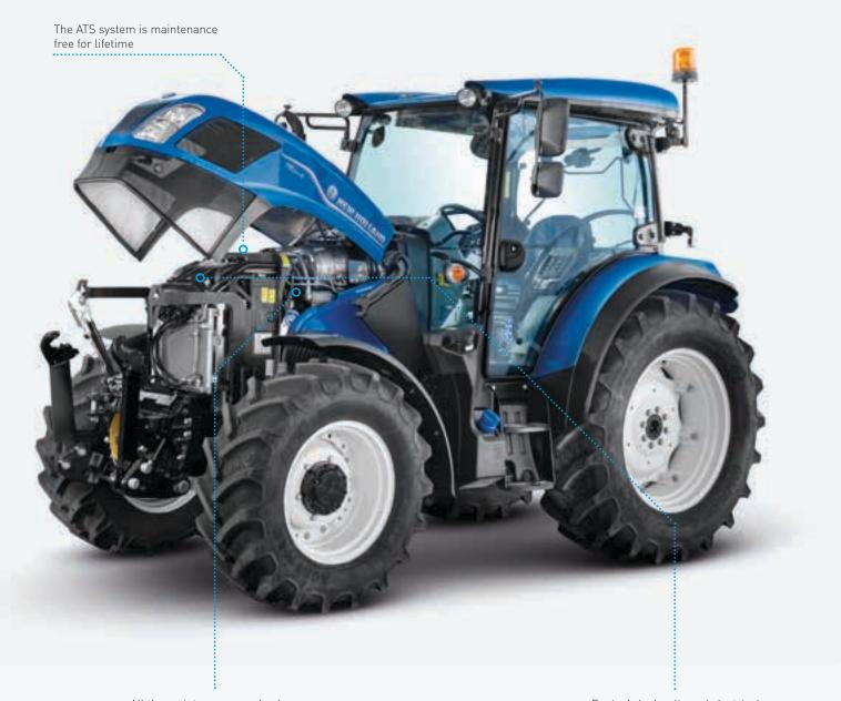
All the maintenance can be done on one side, all service points are on the left side of the engine to make routine servicing easier
