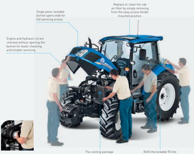
The engine air filter is easy to check, clean or replace, with no need for tools.
